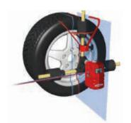
Even if measuring system is not centered to tyre, sensor is still correctly parallel to car.
